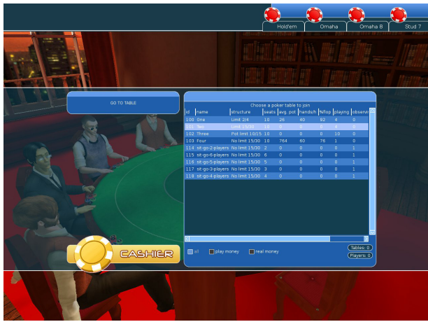
Figure 8: Poker3D as a Metisse compositor: the blue windows contain GTK+ interface elements and are rendered by the Metisse server.
